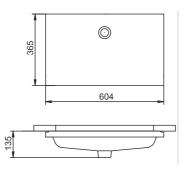
LW542MUNW1 Under Counter Washbasin (w/o Bracket) Size: 530W x 365D x 206H mm
