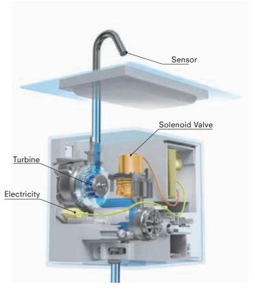
This ECOPOWER touchless faucet uses the flowing water to generate the electricity it needs to operate. There is no need for electrical wiring,
